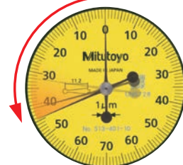
Indicator trackability depends on maintaining gear-train stability
